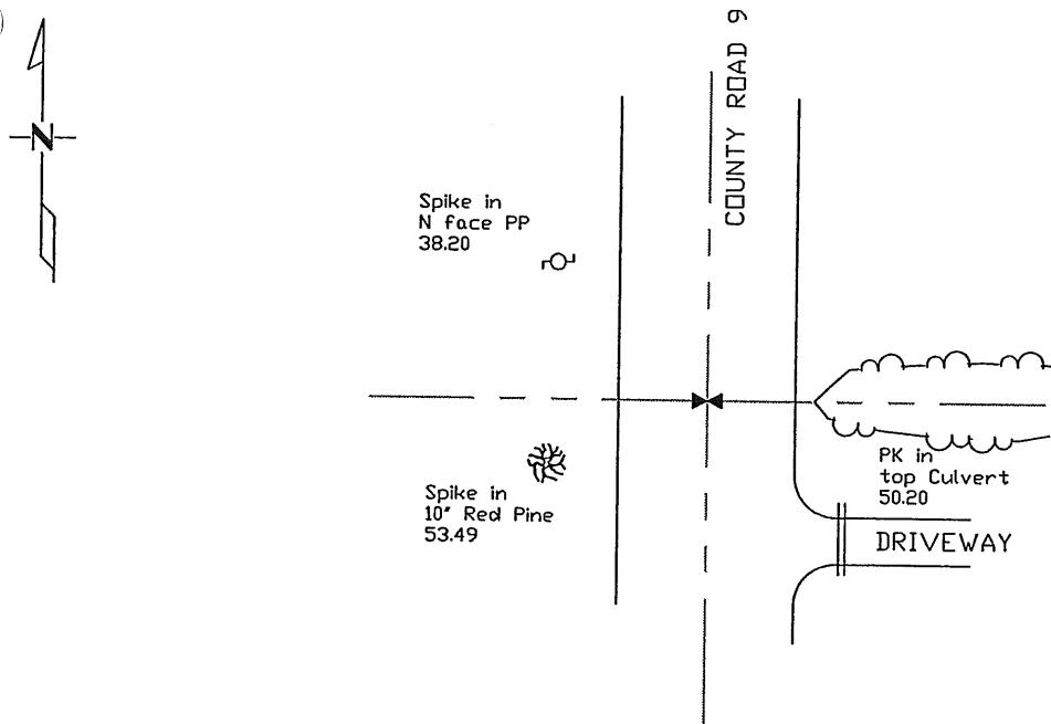
New tree and power pole ties are to the head of a nail with a brass disk marked "Corner Tie".
